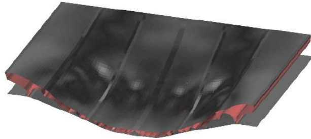
Blast protection using double hull, sandwich structure
